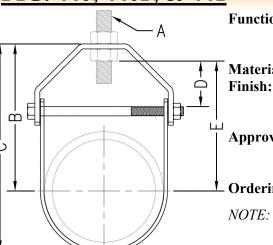
**Function:** Designed for the suspension of non-insulated stationary pipe lines in
